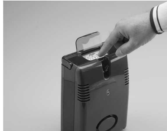
Figure 24: Pressing Flow Selection Button
